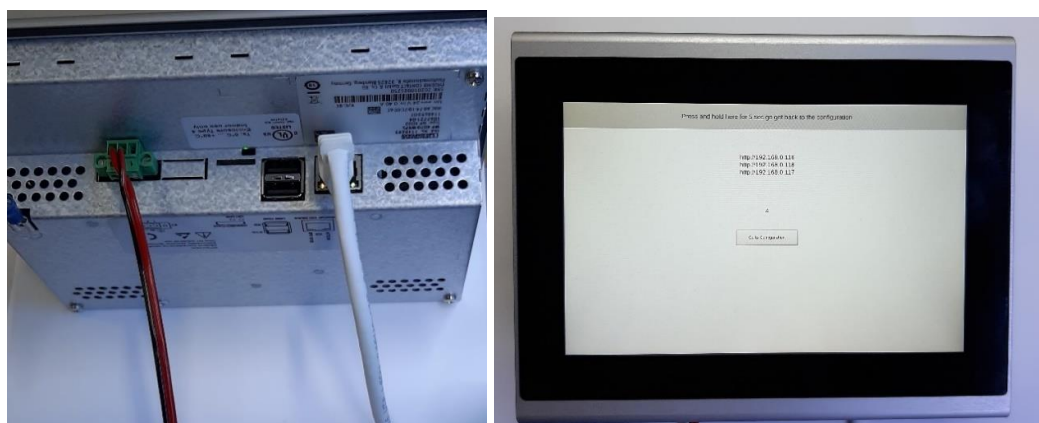
Figure 9 Cable connections to the external display and activation of configuration page during power up.
